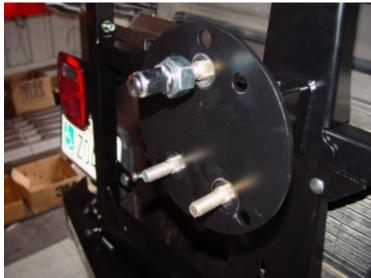
Install the included wheel studs (3) to the wheel hub. They can be installed using an H-frame press or by using a large deep socket and closing it in a bench vise. Once pressed through, the wheel hub can be mounted to the wheel hub extension welded to both the round tube tire carrier and also the antenna post on the square frame unit.
