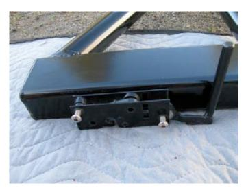
The latch mounts to the bottom side of the swing arm with the supplied 1/4" x 1.25" button head bolts. The arm extension should point in the same direction as the wheel mount (to the rear).
