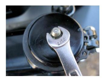
Install snap ring and grease zerk to the spindle assembly. Grease fitting upon completion of tire carrier installation.
